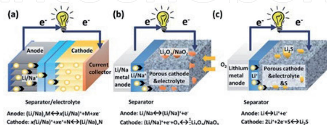
**Figure 4.** Design of (a) Li/Na-ion batteries (*M* represents the anode material, and *N* represents the cathode material), (b) nonaqueous Li/Na-O<sub>2</sub> batteries and (c) Li-S batteries [38].
