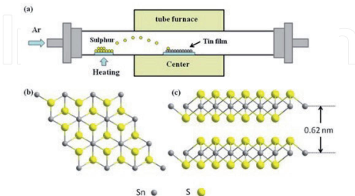
**Figure 2.** (a) Schematic diagram of preparation of SnS<sub>2</sub> film. (b) Top view and (c) side view of the atomic structures of SnS<sub>2</sub> [32].
