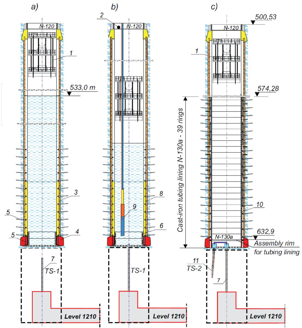
**Figure 2.** The phases of dewatering the sunken shaft section. (a) Shaft flooding. (b) Dewatering of the shaft using a “RITZ” submersible pump, (c) replacing the concrete lining along the 574.3–632.9 m section with a cast-iron tubing lining. Explanations: 1–8, see Figure 1; 9, RITZ submersible pump; 10, cast-iron tubing lining; 11, TS-2 dewatering borehole.
