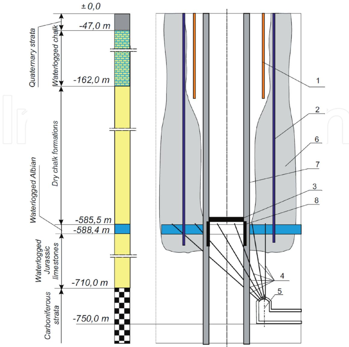
**Figure 4.** Diagram of the S-1.3 shaft sinking using both rock freezing and rock heating. 1, boreholes for rock heating along the 0–180 m section; 2, boreholes for deep freezing along the 0–570 m section; 3, concrete plug above the Albian layer; 4, drainage boreholes in the Albian layer; 5, working with a drilling chamber at a depth of 754 m; 6, frozen rock mantle; 7, final concrete panel lining; 8, cast-iron tubing lining along the Albian formation section.
