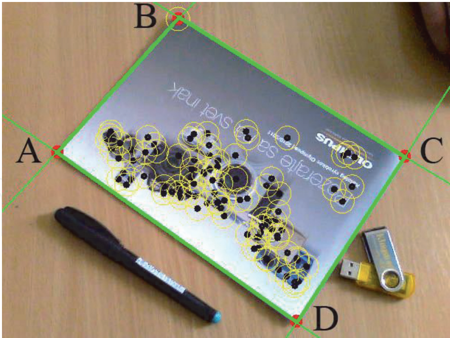
Figure 14. Rectangle ABCD and interest points obtained by SURF method.
