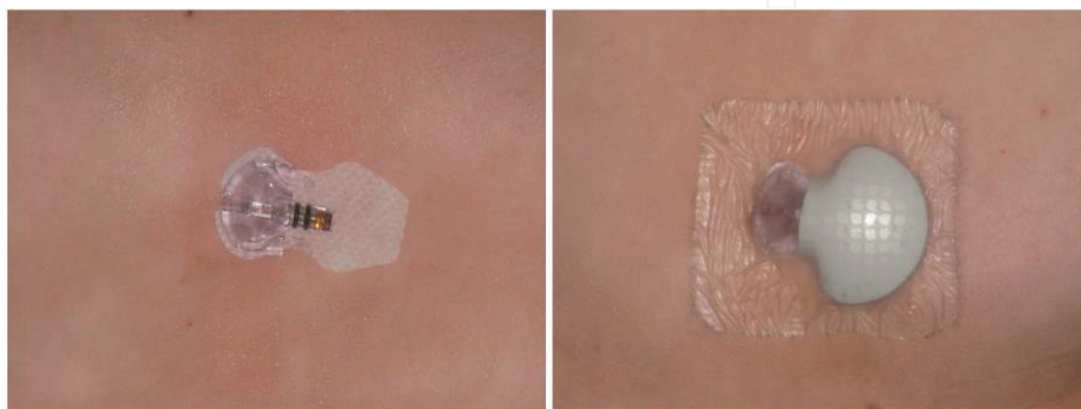
Figure 2. Continuous glucose monitor sensor, before and after attachment of the transmitter. 'CGM set' and 'Continuous Glucose Monitor' by Sara Bassett are licensed under CC BY-NC-SA 2.0.
