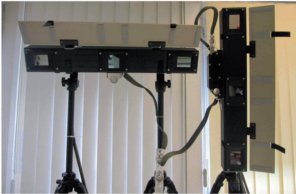
Figure 10. The tracking system (CODA cameras).
