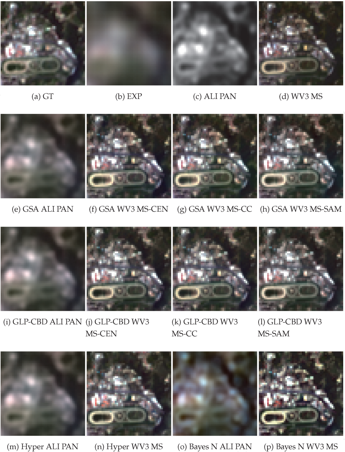
Figure 2. Close-ups of the products achieved by applying the pansharpening algorithms to the RR Agnano dataset (red, green, and blue bands). The resolution enhancement factor is R = 6 (WorldView-3 satellite images courtesy of the DigitalGlobe Foundation). The figure labels indicate the fusion method (see Section 3.3), the high resolution data and the assignment algorithm (see Section 2.1.2), utilized.
