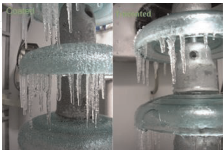
Figure 11. Comparison of the uncoated and superhydrophobic coated sample at -5^{\circ}\text{C} and high humidity [35].
