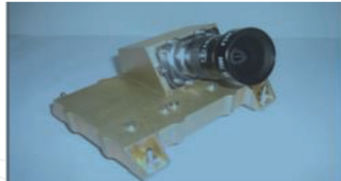
Figure 11. r-vector sensor HS CMOS/SRAM-modular infrared horizon sensor, accuracy, 0.4 deg. ( 2\sigma ).
