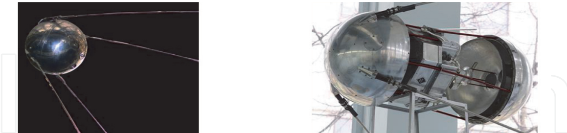
Figure 2. SS-1, assembled (left). Open two semispheres (right).
