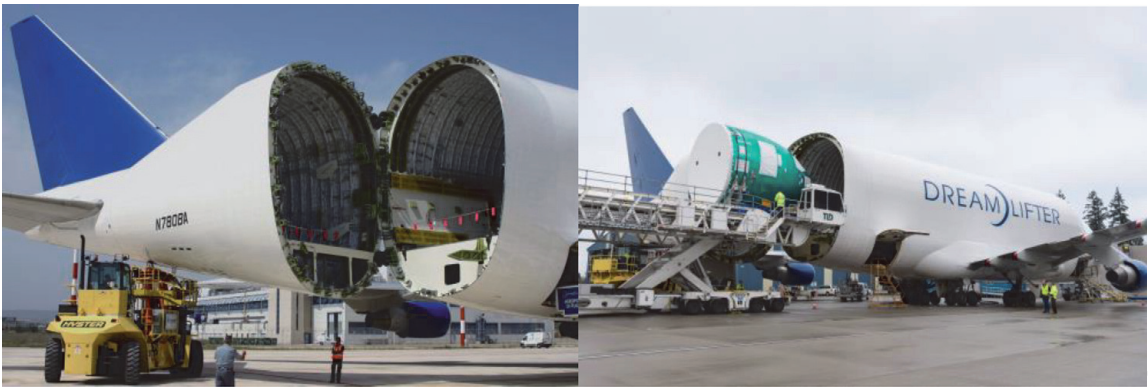
Figure 28. Rear cargo door of “Dreamlifter” B747.
