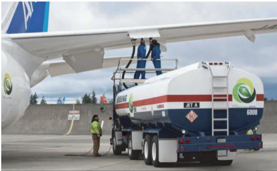
Figure 21. Airplane fueling from the service car—non-rational.
