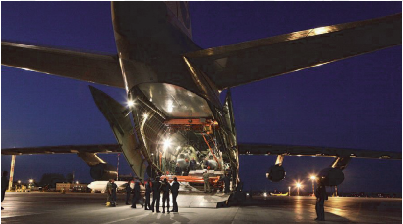
Figure 27. The rear cargo door of the heavy cargo airplane Antonov An-124, night loading procedure.
