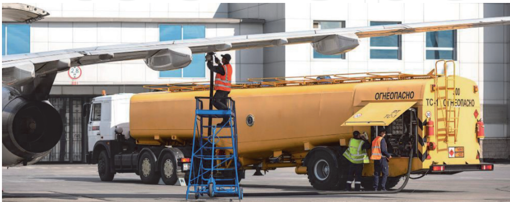
Figure 22. Airplane fueling from the ground stairs.
