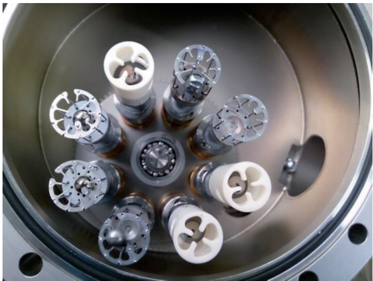
Figure 9. Sample magazine of the parabolic flight facility with eight samples in cups and cages.
