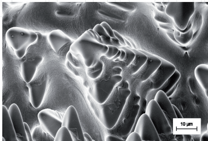
Figure 1. Scanning electron micrograph of the surface of an as-cast \text{Fe}_{99}\text{B}_1 alloy showing the morphology of metallic dendrites. The length scale is indicated by the horizontal bar (M. Kolbe, T. Volkmann, DLR Cologne).
