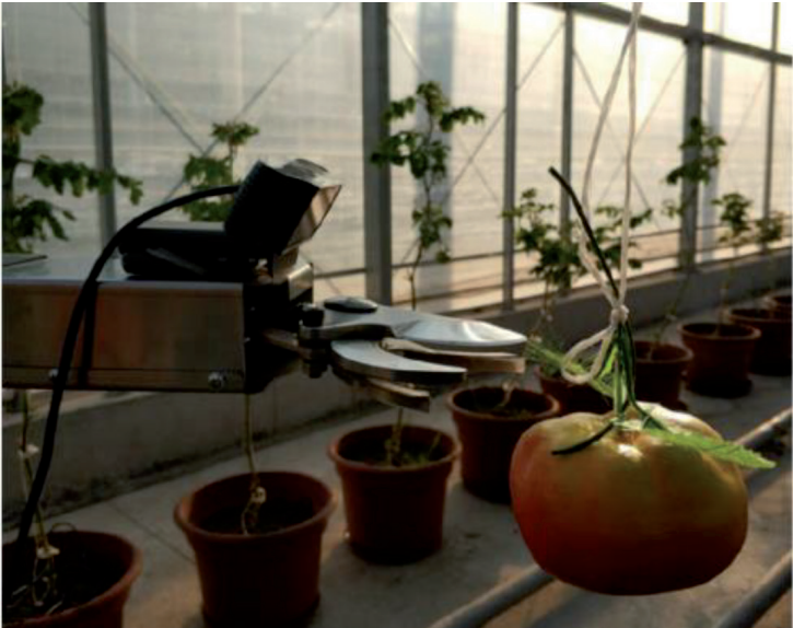
Figure 22. Visual servo program of eye-in-hand.
