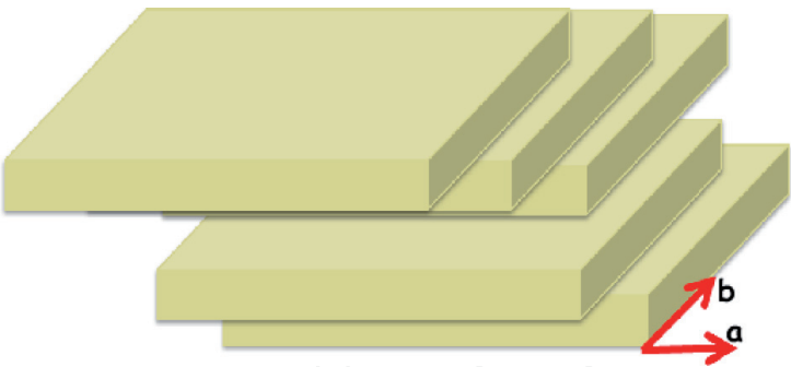
Figure 3. Disordered layers in the vermiculite structure.
