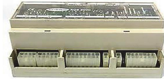
**Figure 2.** Fronius interface to translate the information between serial protocol and data acquisition system with digital and analogical inputs and outputs.
