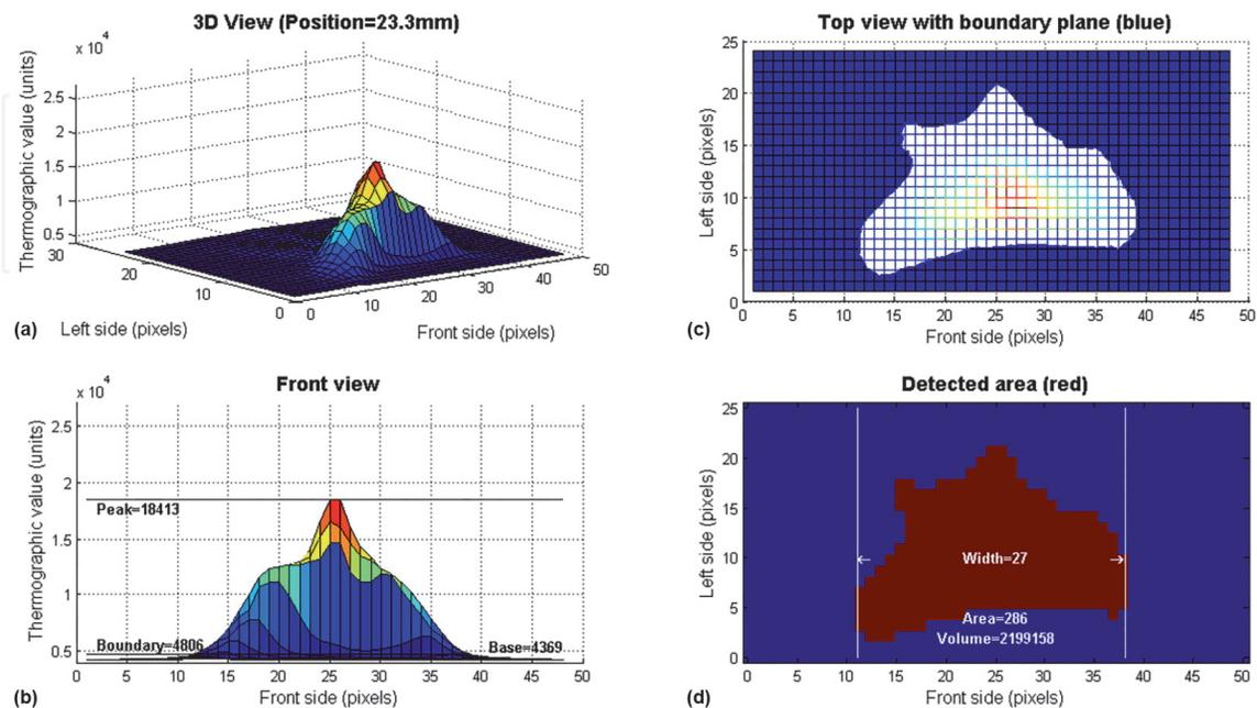
**Figure 18.** Features extracted from an infrared image: (a) three-dimensional curve, (b) front view of the curve, (c) intersection between the boundary plane and three-dimensional curve, (d) and the calculation of the width, area and thermographic volume.
