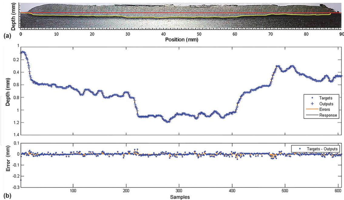
**Figure 19.** Results obtained in the estimation of the weld bead depth in [22]: (a) weld bead depth longitudinal profile and (b) model response and experimental measurements. In the sample axis, each value corresponds to a position in the piece.
