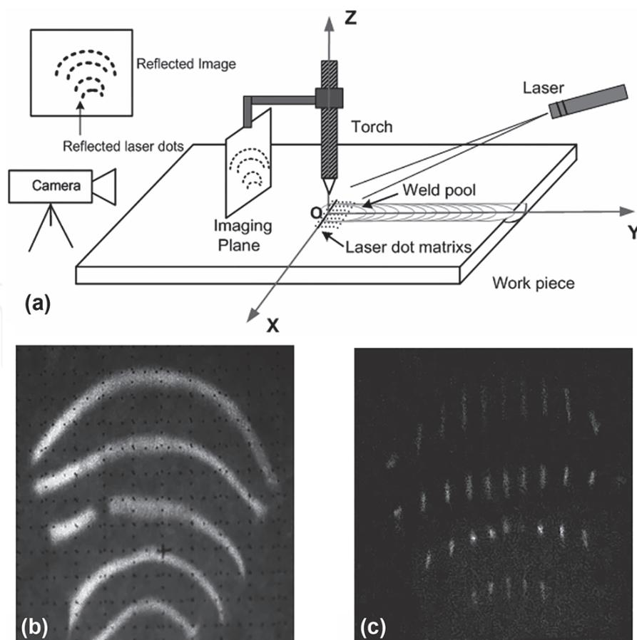
**Figure 11.** Three-dimensional profile of the weld pool surface using structured light and triangulation method: (a) diagram of measure system, (b) reflected image using line laser pattern, and (c) reflected image using dot laser matrix (adapted from [15]).
