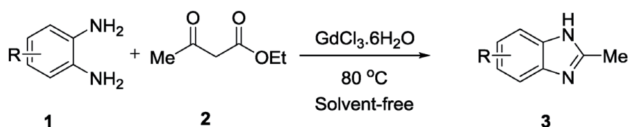
Figure 12. General procedure for synthesis of 2-substituted benzimidazoles.
