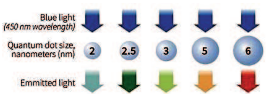
Figure 1. Conversion of the light spectrum into different colors depends on the quantum dot size (image: RNGS Reuters/ Nanosys).
