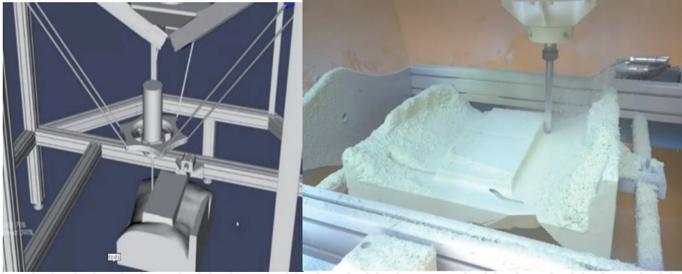
Figure 17. Ortoflex five-axis milling machine based on parallel kinematics.
