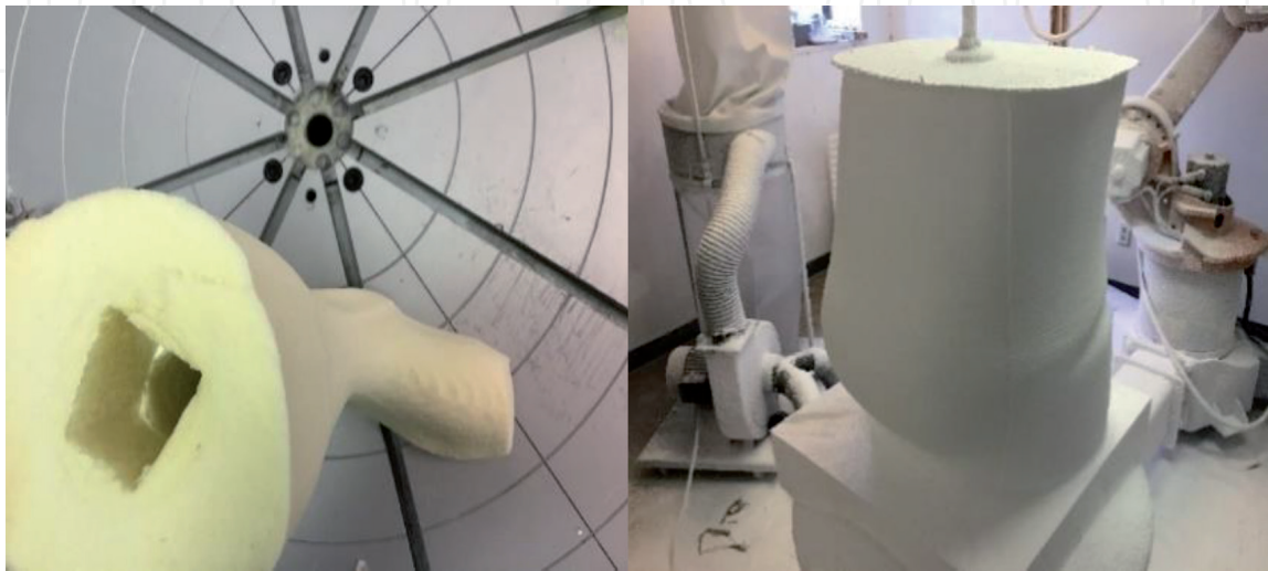
Figure 15. Molds produced from expanded PU foam.
