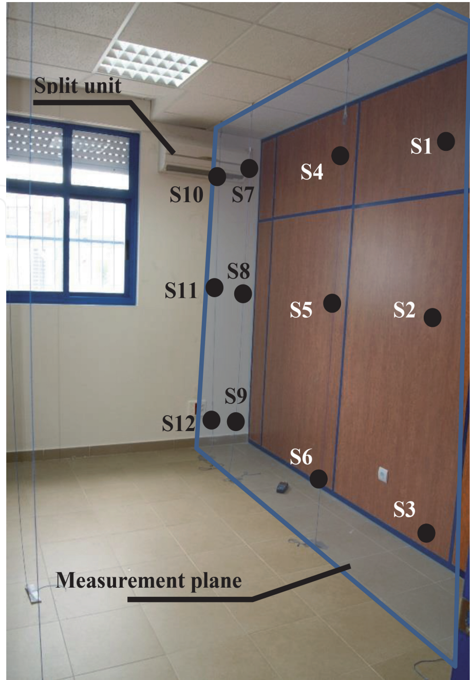
Figure 3. Location of temperature sensors in the experimental office room.
