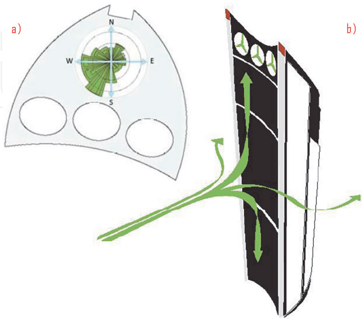
Figure 5. Orientation study based on prevailing wind direction; site plan sketch with wind rose (a) and an illustration of airflow distribution around the tower (b) © BFLS.
