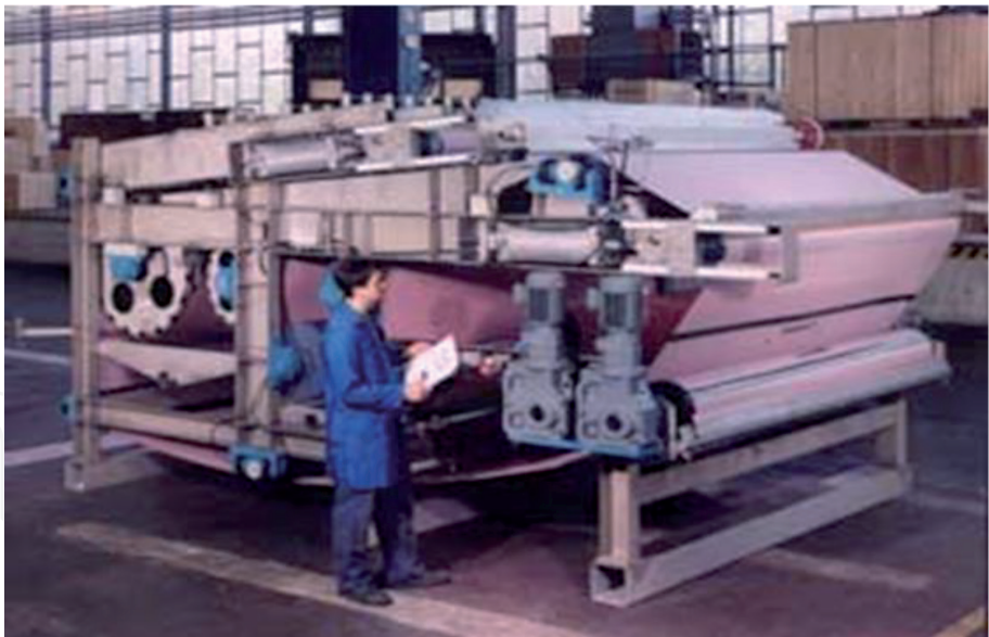
Figure 7. Belt filter press. WWTP-Sabesp, São Paulo, Brazil (source: the author).
