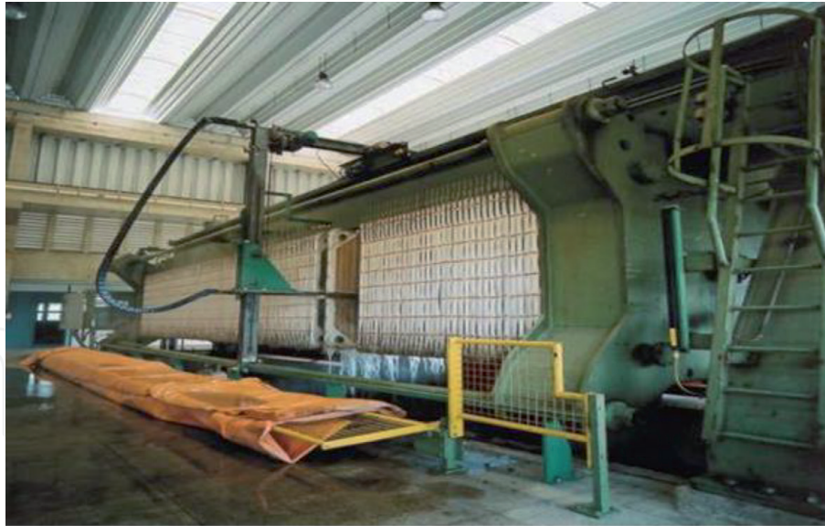
Figure 6. Plate filter press in operation. WWTP-Sabesp, São Paulo, Brazil (source: the author).
