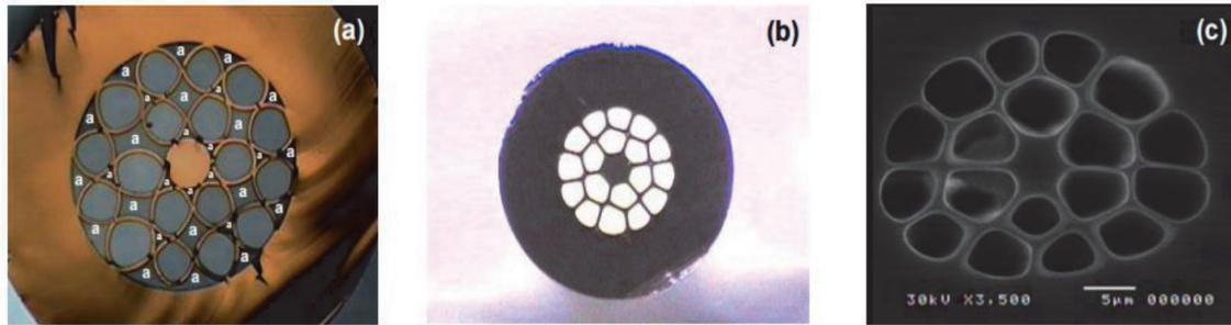
**Figure 9.** (a) Preform with the first clad before eliminating the air trapped. The air regions are indicated with a white “a”. (b) Preform without the air trapped. (c) Scanning electron microscope image of the microstructure fiber [60].
