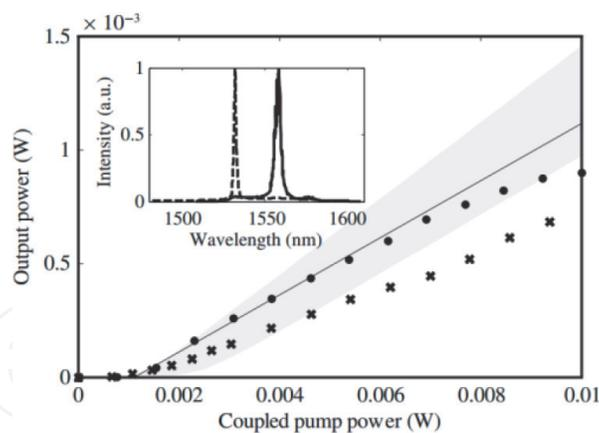
**Figure 8.** Fiber laser output plotted against the coupled pump power for a fiber length of 2.2 m (circles). The figure inset is a plot of the laser output spectrum for 5 mW of coupled pump power into the 1 m (dashed) and 2.2 m (solid) lengths of fiber [59].
