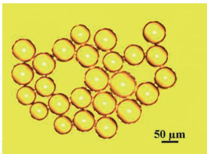
**Figure 26.** Microspheres fabricated by powder floating method.
