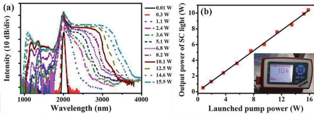
**Figure 22.** (a) Dependence of the measured SC spectra generated from 60-cm-long fluorotellurite fiber on the average power of the 1980 nm femtosecond fiber laser. (b) The dependence of the SC average power on the pump power. Inset: photograph of the power meter when the mid-IR SC laser source is operating at the output power of 10.4 W [52].
