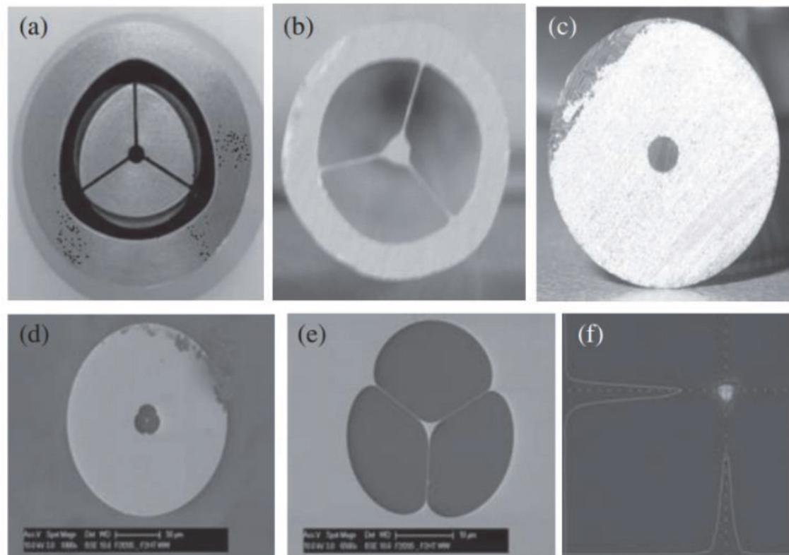
**Figure 7.** Photographs of (a) stainless steel die exit used for the extrusion of the structured preform and (b and c) the extruded structured and jacket preforms, respectively. SEM images of the (d) fabricated fiber cross section, (e) enlarged SEM image of the fiber's core and cladding, and (f) beam profile of the laser mode emitted from the output of the fiber [59].
