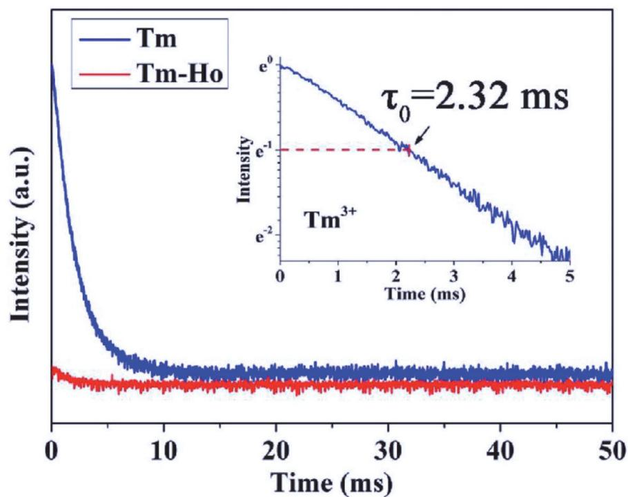
**Figure 32.** Fluorescence decay curves of  $Tm^{3+}$ - $Ho^{3+}$  co-doped and  $Tm^{3+}$ -doped tellurite glass samples at 1.9  $\mu m$ . The inset figure shows that the lifetime of  $Tm^{3+}$  at 1.9  $\mu m$  is 2.32 ms in  $Tm^{3+}$ -doped tellurite glass samples [3].
