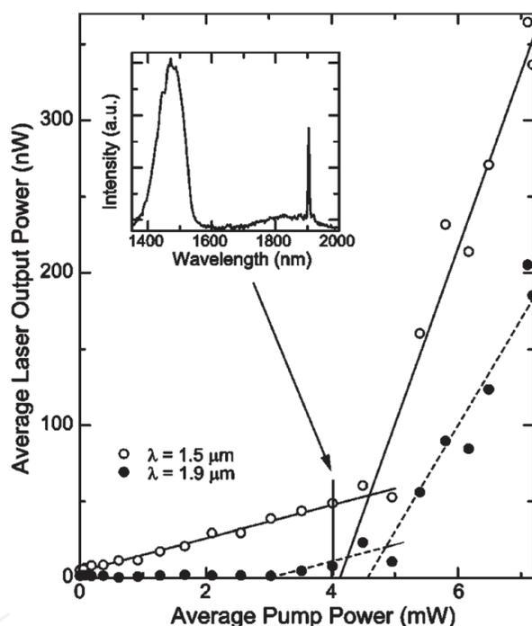
**Figure 30.** Average laser output power against average pump power for a  $\text{Tm}^{3+}$ -doped tellurite microsphere laser. (Inset) Laser emission spectrum at average pump power of  $4.0 \text{ mW}$  [101].
