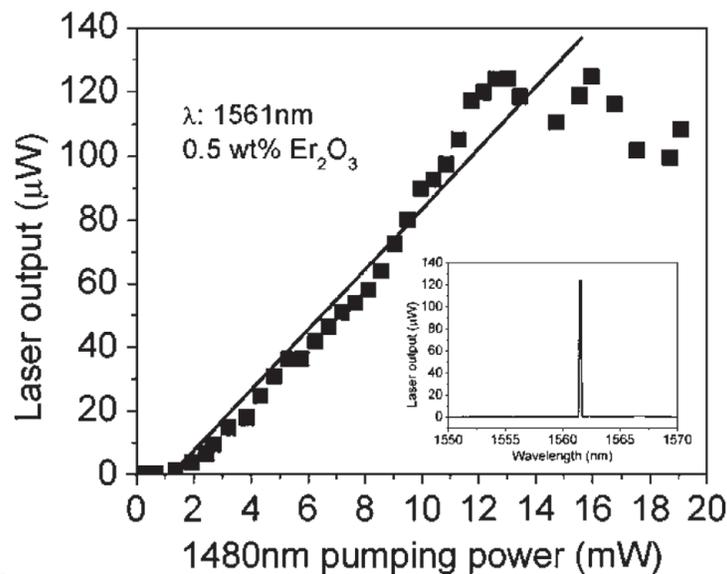
**Figure 28.** The microsphere laser pumped by a 1480 nm laser. The  $Er_2O_3$  doping concentration is 0.5 wt%, and the diameter of the microsphere is 32  $\mu m$ . The maximum output power is 124.5  $\mu W$ . The inset shows the single-mode profile of this L-band microsphere laser [97].
