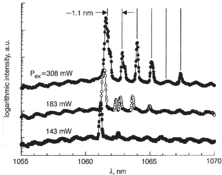
**Figure 27.** Emission spectra for  ${}^4F_{3/2} \rightarrow {}^4I_{11/2}$  transition of  $Nd^{3+}$  ions in tellurite glass microsphere at various pumping powers [96].
