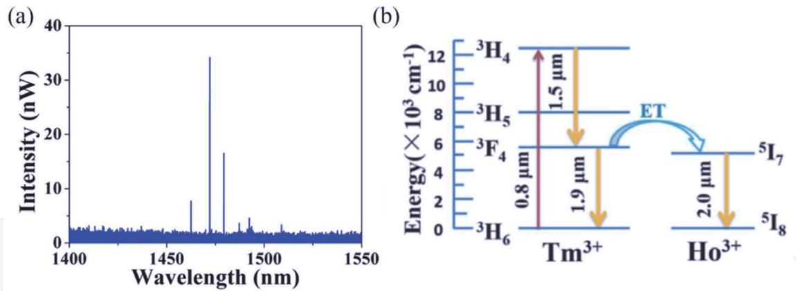
**Figure 31.** (a) Laser emission spectrum from the  $\text{Tm}^{3+}$ - $\text{Ho}^{3+}$  co-doped microsphere when the pump power was set to 2.5 mW. (b) Energy level diagram and energy transfer model in tellurite glass [3].
