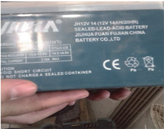
Figure 5. The used battery of 12VDC and 14 amp.hr.
