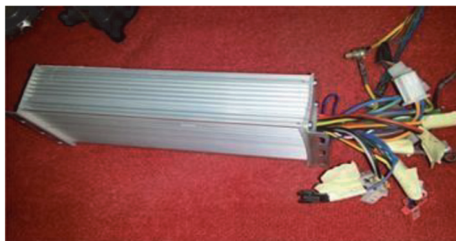
Figure 4. The DC to three-phase voltage inverter used.
