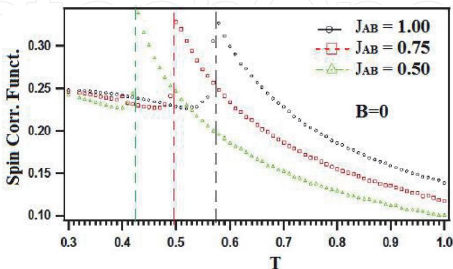
**Figure 10.** Correlation function vs. temperature for a two-dimensional thin film. Spontaneous magnetization is marked by discontinuity in it (this figure is reproduced with permission from Singh [28]).
