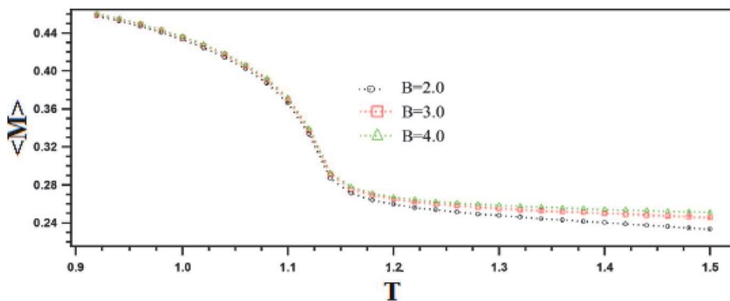
**Figure 15.** Magnetization vs. temperature for magnetically striped system. Only one region experiences the presence of external magnetic field as illustrated in Figure 12(a). This simulation is done for simple cubic lattice with semi-infinite free boundary conditions (the figure is reproduced with permission from Singh [29]).
