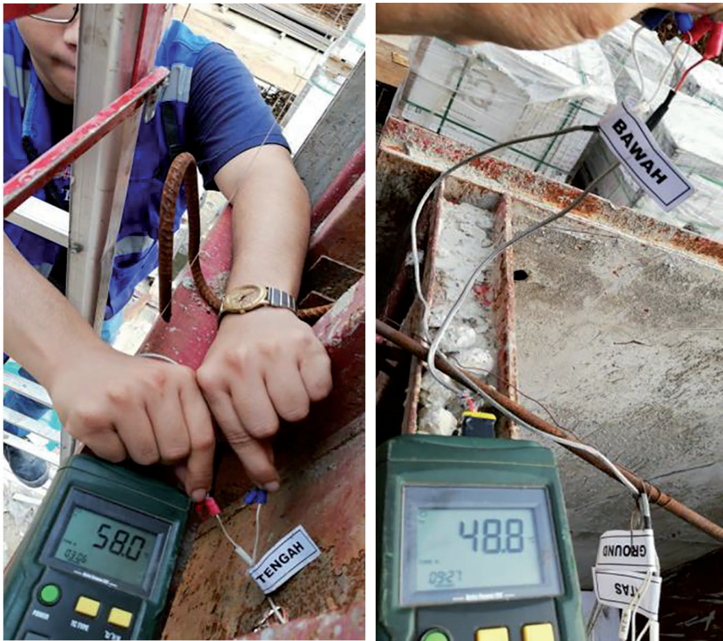
Figure 18. Bioconc LHC mock up thermocouple monitoring.
