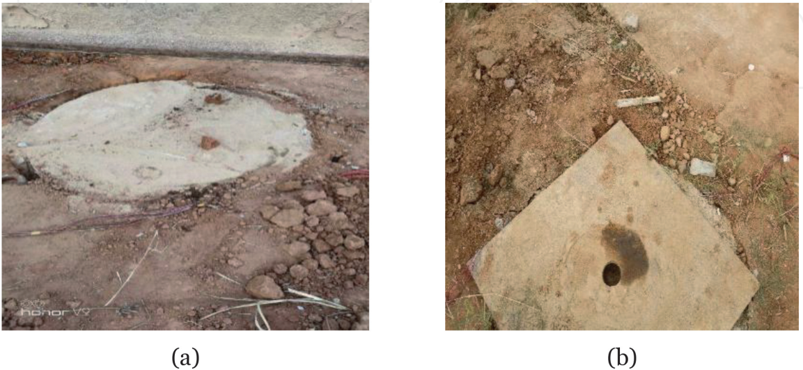
Figure 16. Failure modes of concrete piers. (a) Soil around the pier when the precast pier foundation of recycled compound concrete was destroyed, (b) soil around the piers when the foundation of the cast-in-place ordinary concrete was destroyed.
