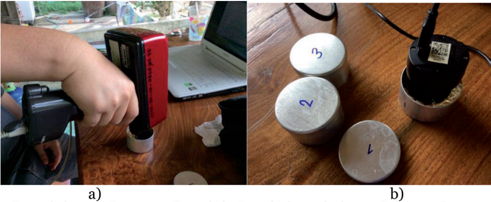
Figure 4. Scanning of wood chips using portable NIR spectrometer (a) NIR-gun and (b) MicroNIR spectrometer.
