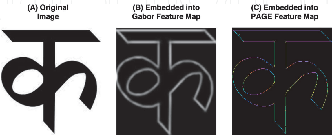
Figure 8. Comparison to Gabor feature extractors: Features detected using Gabor do not have inherent spatial feature localization. With PAGE, the features are more sharper as the bandwidth of the response is determined by the input image dimension.
