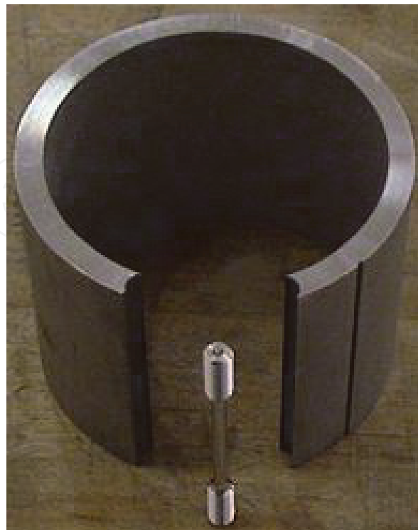
Figure 5. Axial tensile specimen extraction from wall material.
