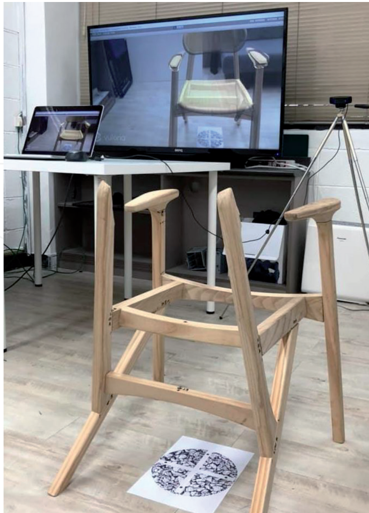
Figure 5. AR can contribute to the comparison between the physical and the virtual shapes in the furniture prototyping process.
