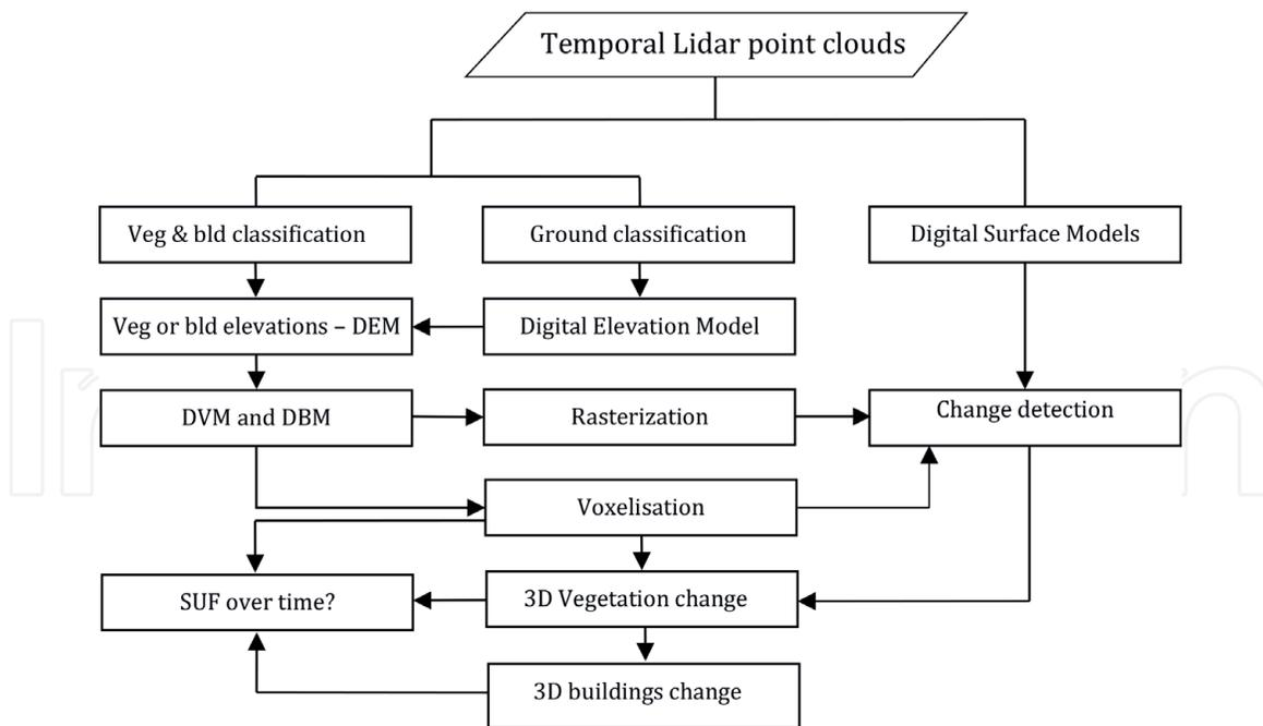
**Figure 3.** The flowchart of the proposed procedure of airborne lidar data processing for the calculation of 3D metrics of sustainable urban form. Note: UFS: Urban form sustainability; DBM: Digital building model; DVM: Digital vegetation model; bld: Building; veg: Vegetation.
