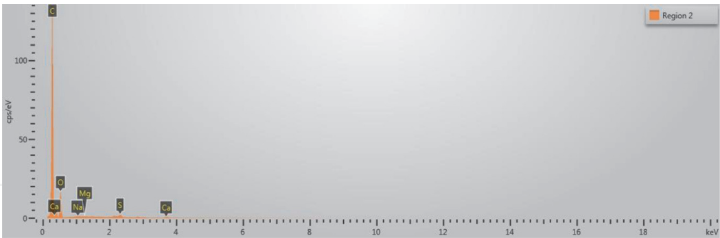
Figure 4. Energy dispersive X-ray spectroscopy result of the highly calcified region 2, shown in Figure 2 .
