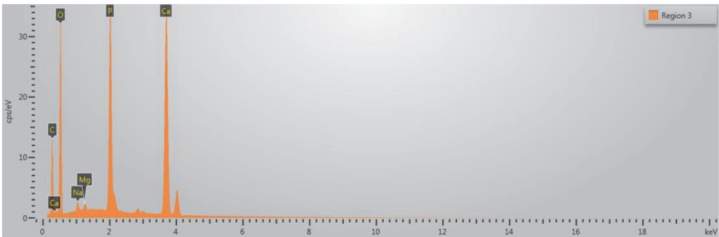
Figure 5. Energy dispersive X-ray spectroscopy result of the highly calcified region 3, shown in Figure 3 .
