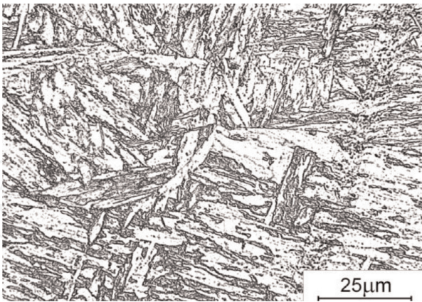
Figure 36. FB2-BM microstructure in as-delivered state, before ACT, LM.
