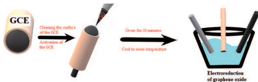
Figure 1. Process of modifying the surface of the glassy carbon electrode.
