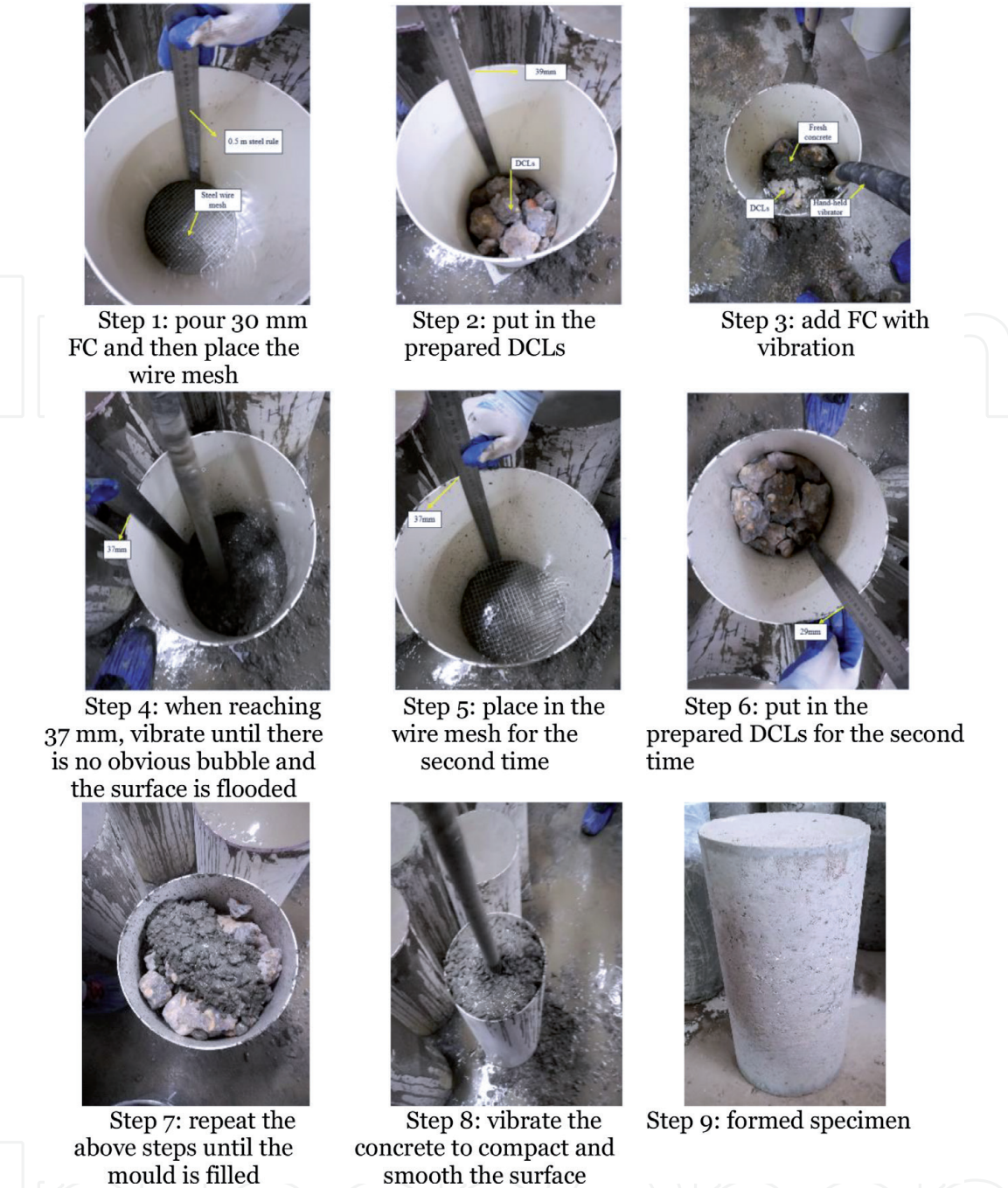
Figure 3. Construction process of specimens.
