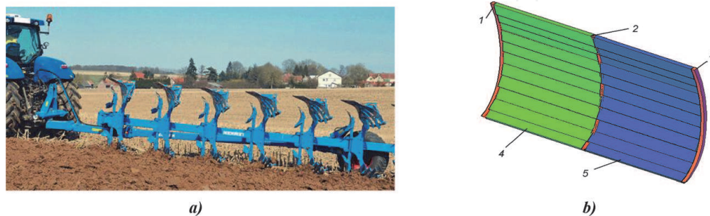
Figure 3. Elemental (plates) construction of plow (a) and bulldozer* (b) moldboard's surface: 1-right, 2-middle and 3-left guiding frames, 4-right and 5-left formative plates (*construction offered by author).
