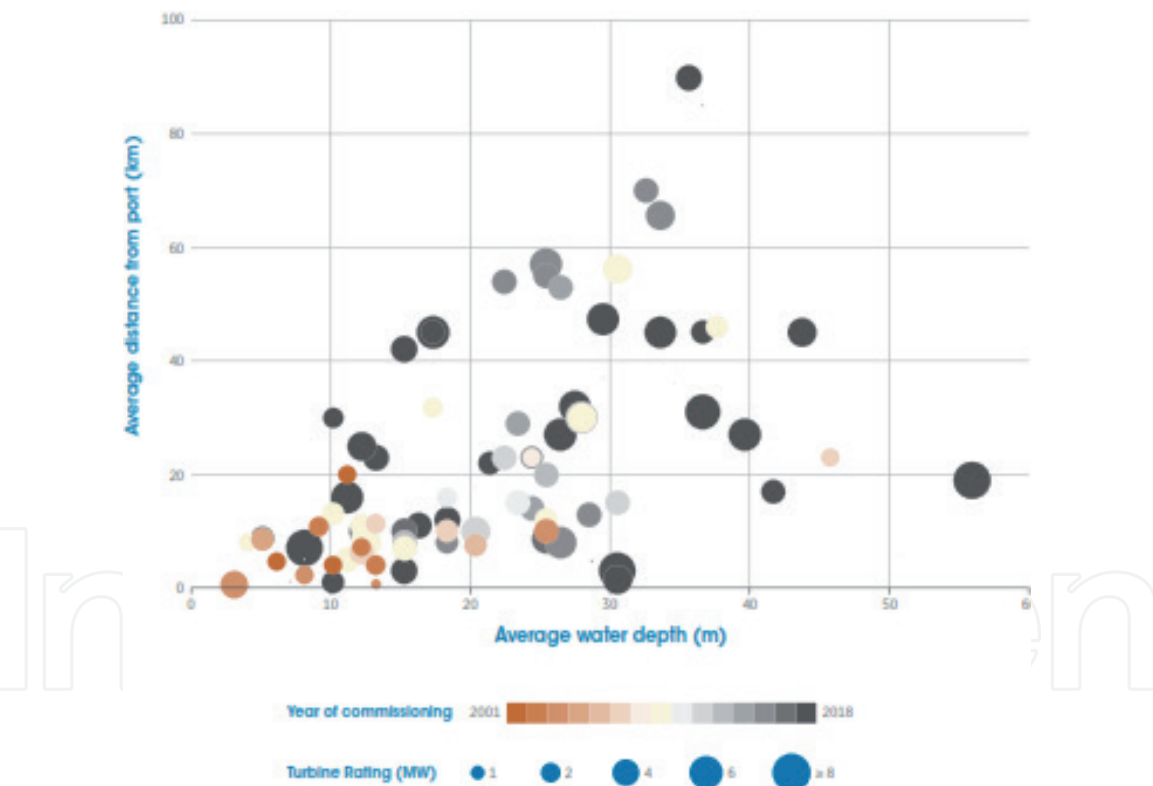
Figure 28. Average distance from port and water depth for commissioned offshore WE projects, 2001–2018 [39, 40].
