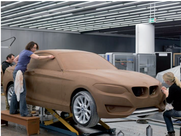
Figure 6. Clay modelling in full scale (source: https://i.pinimg.com/originals/40/fa/22/40fa22a8d8120cceed06deeb0302db12.jpg ).
