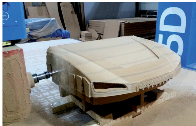
Figure 16. High-speed CNC machining of car body (source: cnc-modelle.com).
