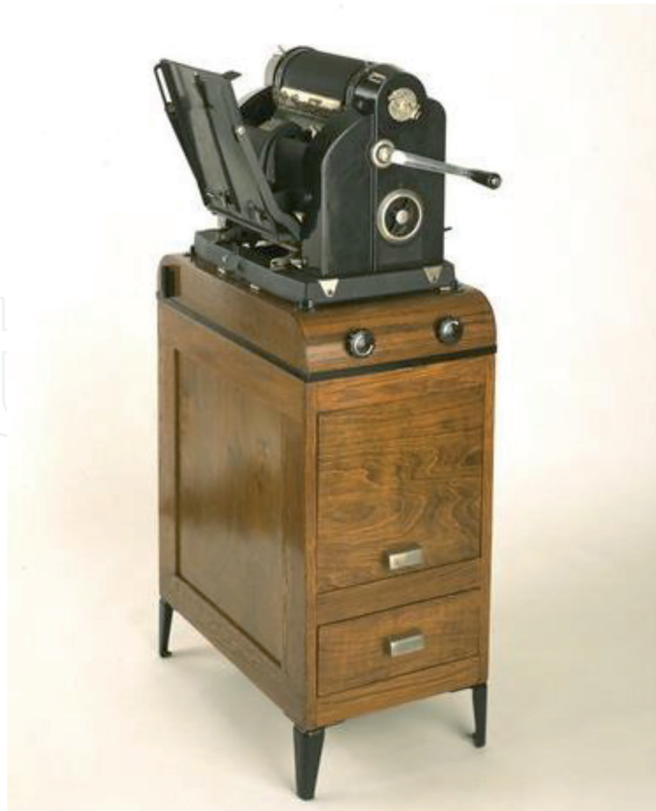
Figure 3. Lowey's redesign of Gestetner duplicator; first use of clay to model the form (source: https://collections.vam.ac.uk/item/O322014/gestetner-duplicator-duplicator-lowey-raymond-fernand/# ).
