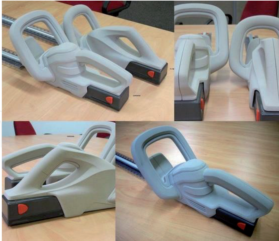
Figure 9. Foam models to check form and ergonomic fits (source: https://www.pinterest.com/pin/289497082275373127/ ).
