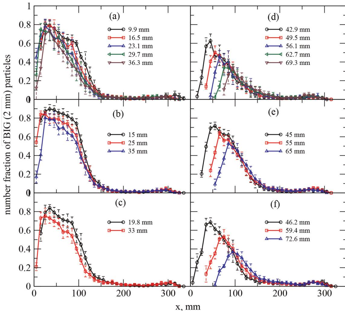
**Figure 8.** Profiles of number fraction of big (2 mm) particles along the flow direction,  $x$  (mm) across the depth in the flowing layer,  $y$  (mm) for equal % of mixture. Volume of pouring (a) 100, (b) 150, and (c) 200 g for top region and similarly for bottom region (d), (e), and (f). Height of the divider from the bottom ( $h$ ) is: 22 cm. Error bars show the standard deviation over eight experiments.
