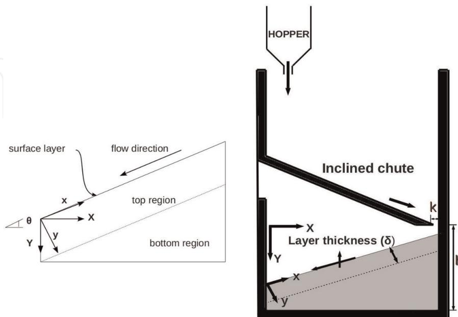
**Figure 3.** Schematic view of heap formation, comprising top and bottom regions (left) along with setup used (right). The coordinate system shows  $x = 0, y = 0$  at the low end of the top surface of the pile. The coordinate system employed in the analysis is shown (left).
