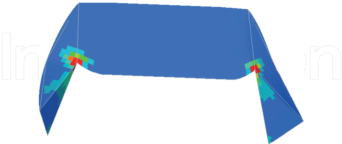
Figure 15. Frequency domain modal superposition damage result plot. Maximum damage = 92.
