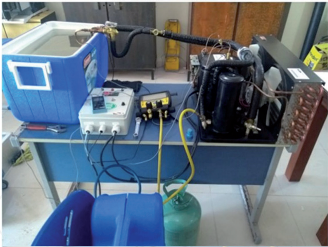
Figure 1. Bench tests with chiller mounted by ClimaTConT.
