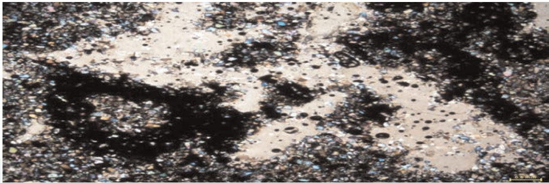
Figure 1. A fairly porous typical oil layer drilled from 3572 m and synthetic sandstone with less percentage of fine crystals of anhydrite, dolomite cement, and sub-round/fossil patches. This rock is associated with small ooids in the middle and intraclasts on all sides which have been poorly sorted. The porosity type is fracture and enormous vugs ( \phi = 16\% ) containing the oil.
