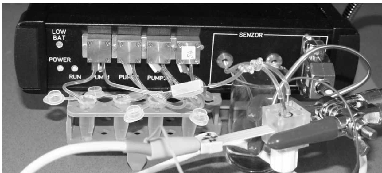
Fig. 5. The amperometric immunosensor detector ImmunoSMART. In the left part of the front pannel, four miniature peristaltic pumps are connected to minitubes with bioreagents. The flow-through cell fixed in the holder contains the exchangeable screen-printed immunosensor.
