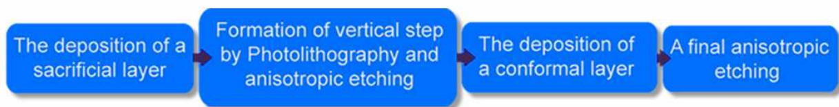
Fig. 1. Step Requirement for fabricating Nanowire using SPL
