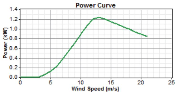
Figure 6. Wind turbine power curve.
