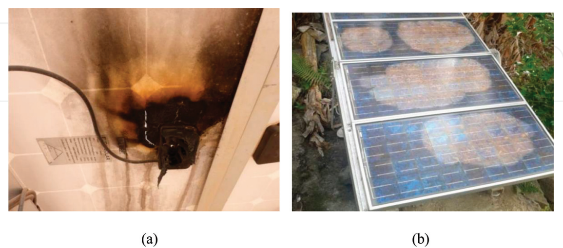
Figure 6. (a) PV junction box and (b) delamination and discoloration.
