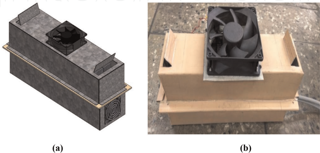
Figure 5. Thermoelectric air conditioning system.
