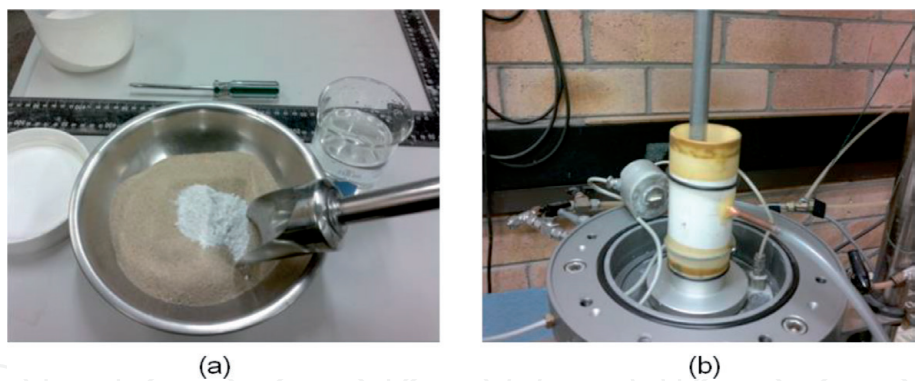
Figure 15. Procedure of (a) mixing and (b) molding bio-cemented samples for triaxial test.
