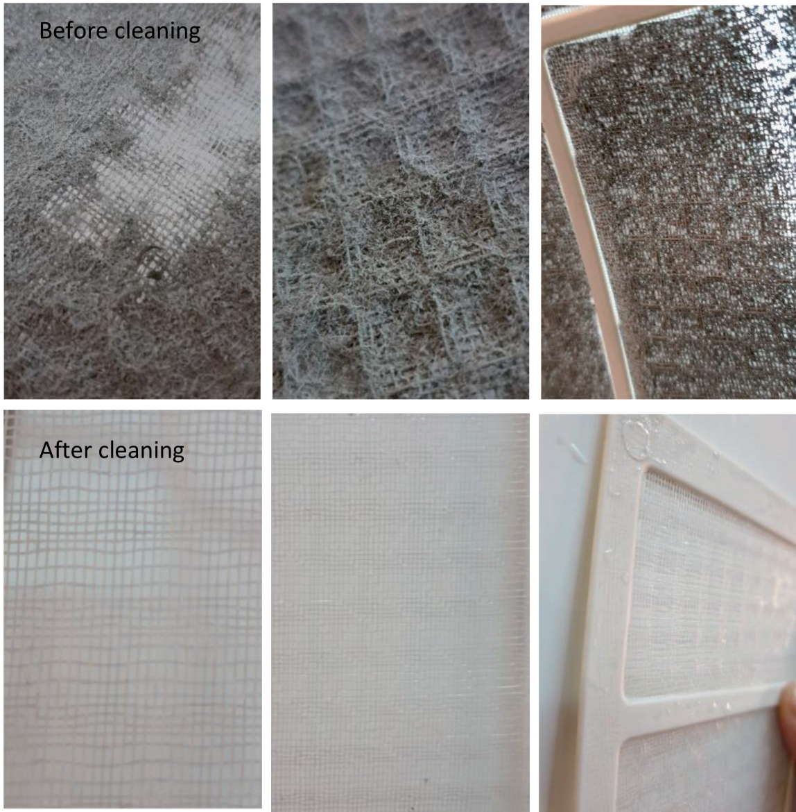
Figure 1. Accumulated dust on discarded polyester filters.
