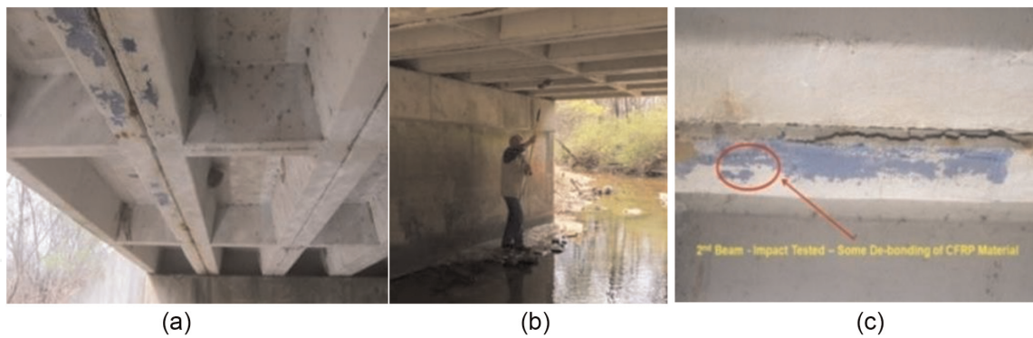
Figure 5. Creasy Springs Road bridge—impact testing on channel beams. (a) Second and third beams, (b) testing fourth beam, and (c) CFRP de-bonding second beam.
