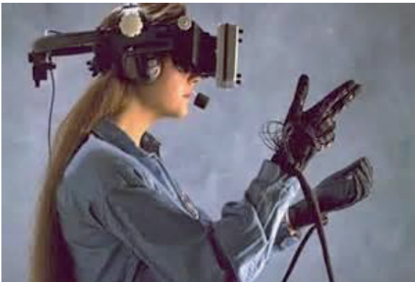
Figure 2. Immersive virtual reality; head mounted displays (HMD) and data gloves [5].
