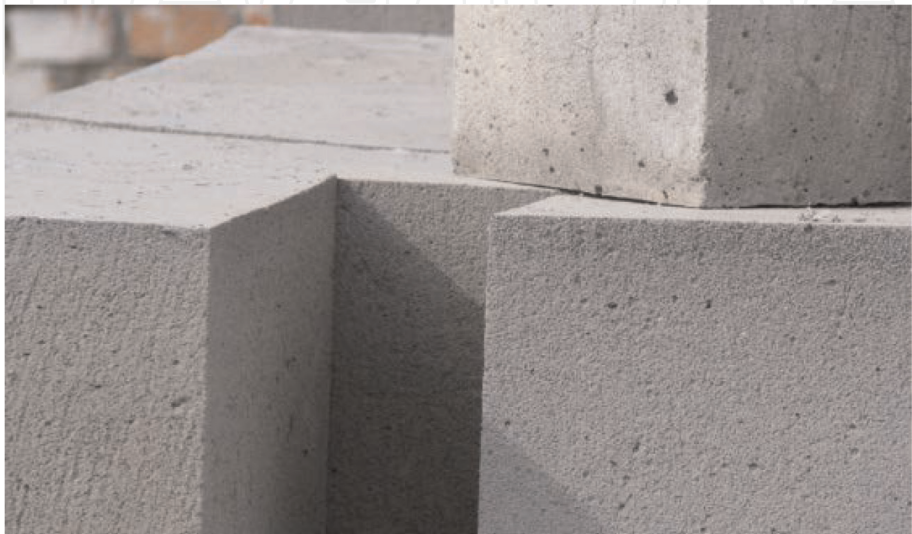
Figure 15. Foam concrete products based on the stabilized foam and NaCl additives.
